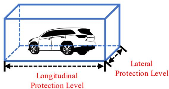
Figure 7 Bounding box definition for autonomous vehicles
