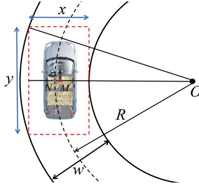
Figure 8 Bounding box geometry in a turn
