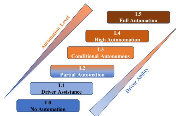
36 Figure 1 Society of Automotive Engineers (SAE) levels of road vehicle autonomy
